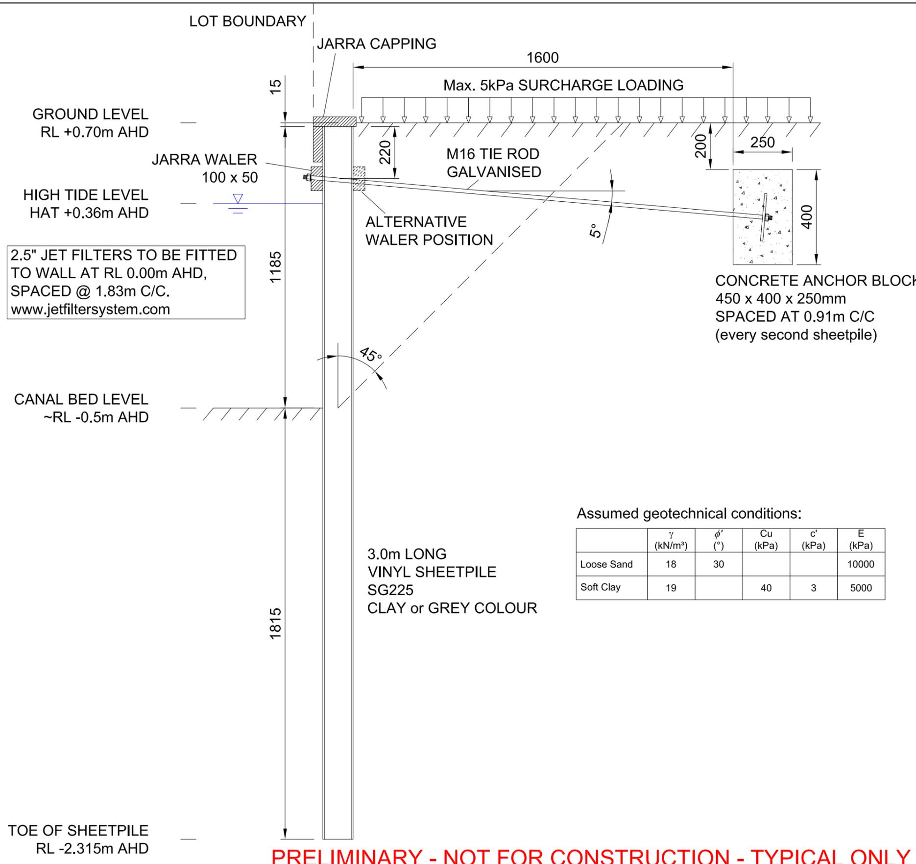
2.5" JET FILTERS TO BE FITTED TO WALL AT RL 0.00m AHD, SPACED @ 1.83m C/C. [www.jetfiltersystem.com](http://www.jetfiltersystem.com)
